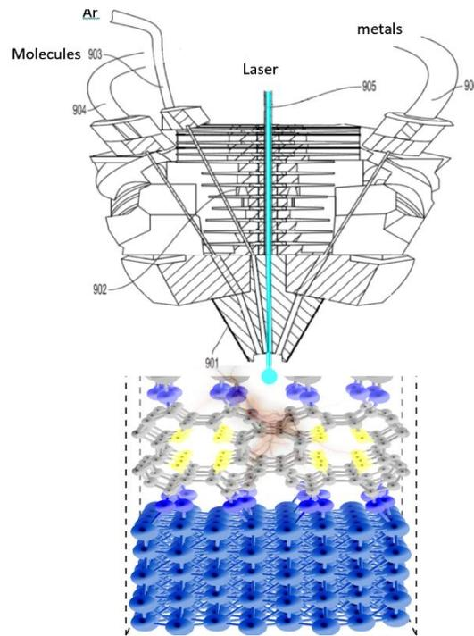
Schematics of creating 3D structures using molecular SAM with a Multi orifices extruder.
