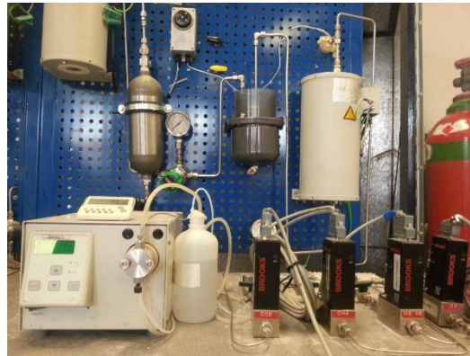
Fig 1. Experimental apparatus used for catalytic reaction activity test
