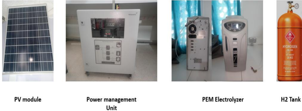
Fig. 1. Hydrogen system components
